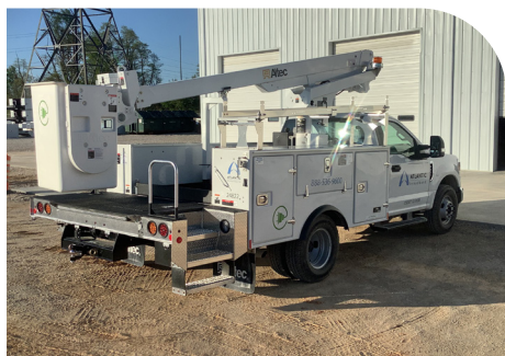
Breezeline bucket truck that uses a Jobsite Energy Management System (JEMS) to avoid running the engine when operating the bucket lift.
